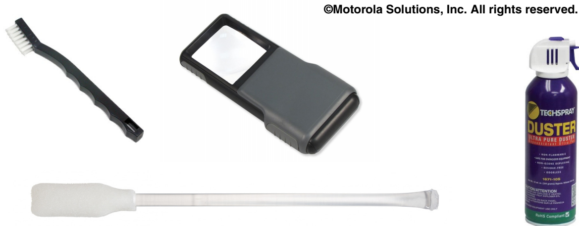
Figure 9-44 Examples of Connector Installation Cleaning Supplies
