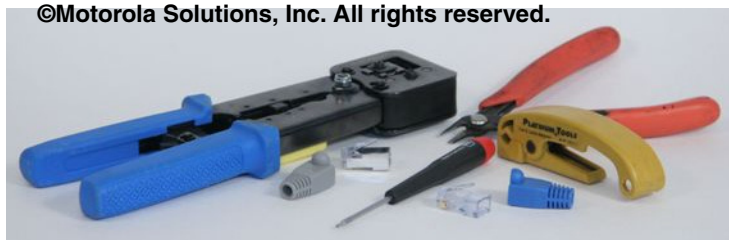
Figure 9-32 Tools for Network Cable Connector Installation
