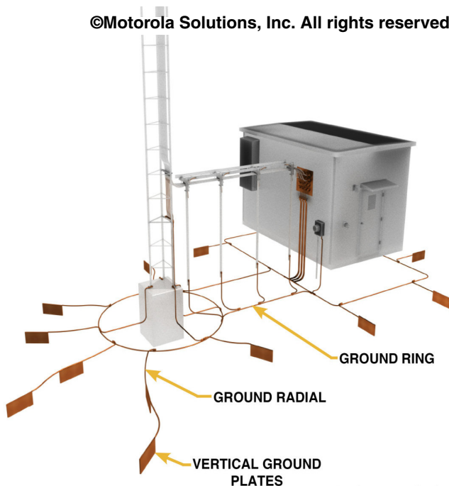
Figure 4-119 Installation of Ground Plates in Shallow Topsoil Conditions
