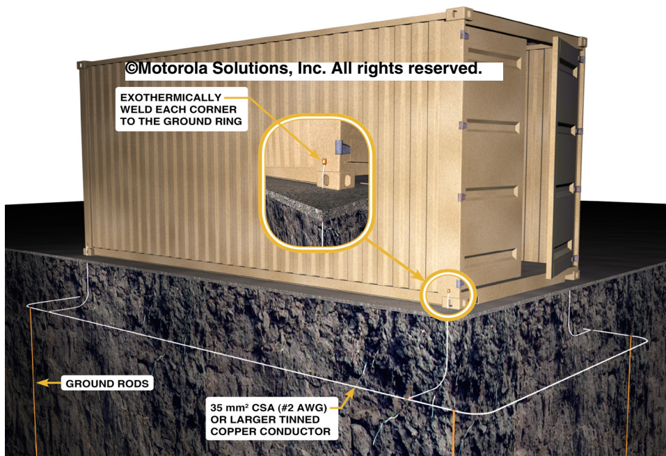
Figure 4-110 Grounding of Metal Shipping Containers
