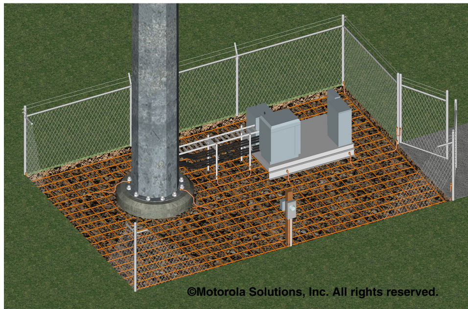
Figure 4-31 Typical Wire Mesh Installation at Site with Limited Space (Ground Cover Not Shown)
