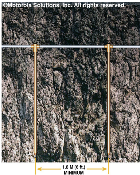
Figure 4-12 Parallel Ground Rod Installation
