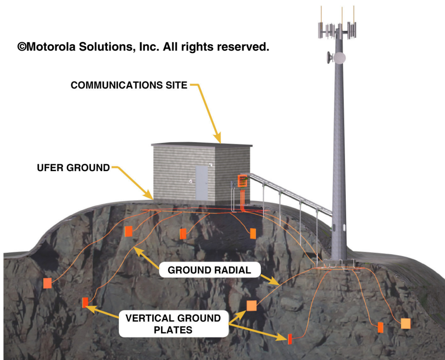
Figure 4-117 Installation of Radials and Ground Plates on Stone Mountaintop Site or Site with Shallow Topsoil
