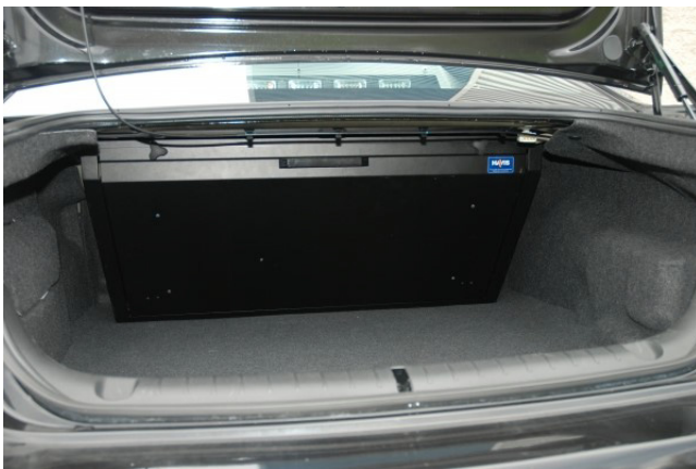
Figure G-3 Examples of Trunk Fold Away Mounting System (Photo Courtesy of Havis)
