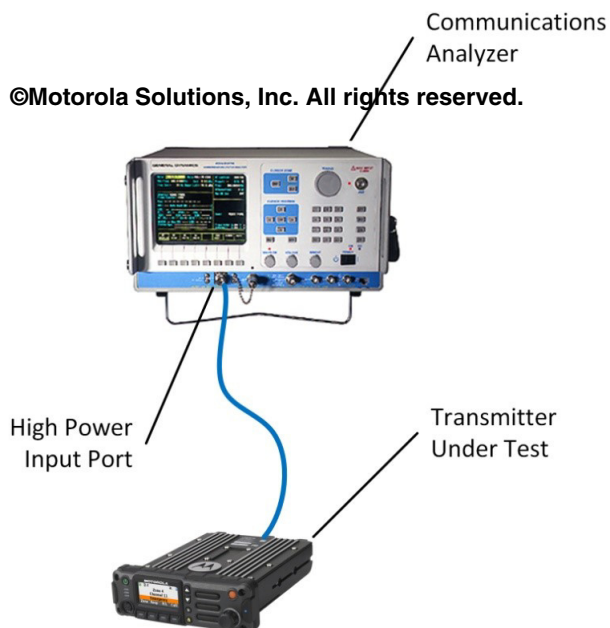
Figure G-39 Example of Configuration for Transmitter Noise Test
