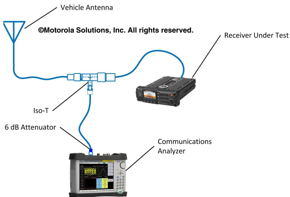
Figure G-38 Configuration for Measurement of Effective Receiver Sensitivity with Vehicle Antenna
