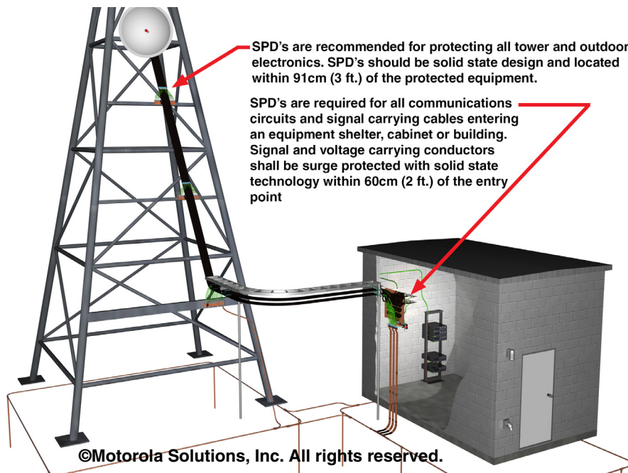
Figure 7-24 SPD Locations for Broadband Wireless Radios
